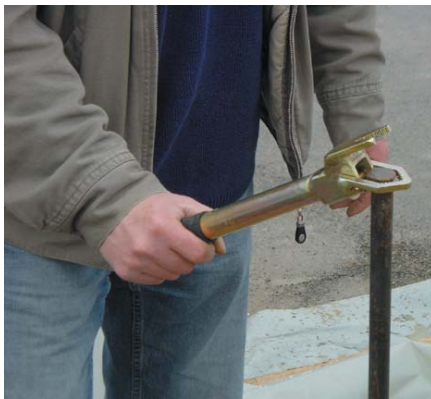
Pin Extractor ENZ is simply put over the top end of the pin.
