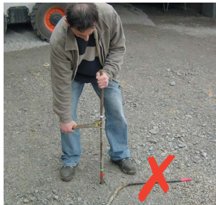
When lifted up, the V-shaped clamping system locks to the pin. Now pulling and turning movements to loosen the pin, can be executed without any real physical effort.
